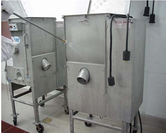
Power wash grinder.
